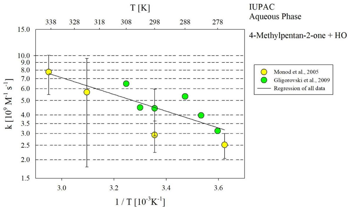
T-dependent rate constants for the reaction of 4-methylpentan-2-one with HO radicals in aqueous solution. All data given in the plot have been used for regression.
